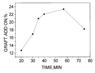
**Figure 3** Relation between time of reaction and graft add-on.
