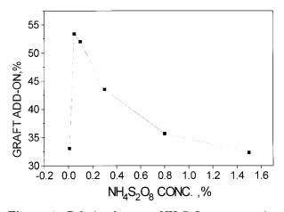
Figure 1 Relation between  $NH_4S_2O_8$  concentration and graft add-on.
