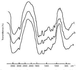
**Figure 6** Infrared spectra: (a) control woolen fabric; (b) grafted wool fabric with graft add-on of 14.14%; (c) grafted wool fabric with graft add-on of 31.74%.
