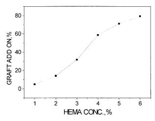
Figure 2 Relation between HEMA concentration and graft add-on.
