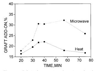
**Figure 5** Relation between time of reaction and graft add-on by means of microwave and heat.
