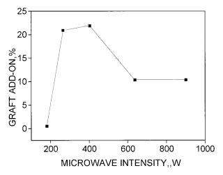
**Figure 4** Relation between microwave intensity and graft add-on.
